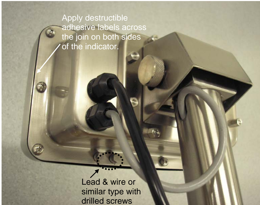
Showing Typical Sealing Methods
